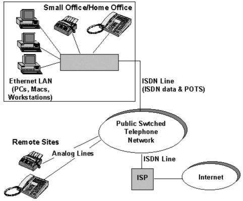
A schematic of how the Hypertec ISDN Router is used is shown in Figure 0-2 A Hypertec ISDN Router Application.
